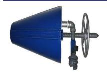
Our **Blow Cones,** Manufactured by Powerhowse Electric have 3 grooves and be used to blow either 12mm blowing tape, 3mm or 6mm rope. We recommend that you block the 2 grooves not in use by filing the gaps with blue tac or chewing gum to stop air for escaping whilst blowing.
