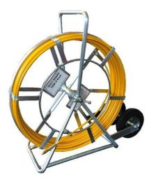
**100M X 8MM** Available in 100m or 125m, for ducts up to 100mm. Steel frame and tension braked, wheels for easy mobility, stand-up or laydown. Trace wire (TW) available.
