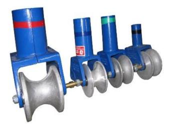
**Note:** To get the best size for your job you will need to know the Internal Diameter (ID) of your Duct/Conduit, this will determine which Bellmouth Roller to use by its Outside Diameter (NECK OD)
